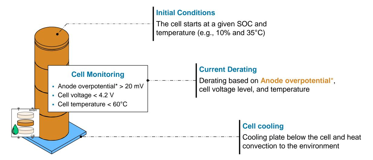
\*The anode overpotential is the electrostatic potential vs. the Li reference. It has been implemented by modifying the source code
